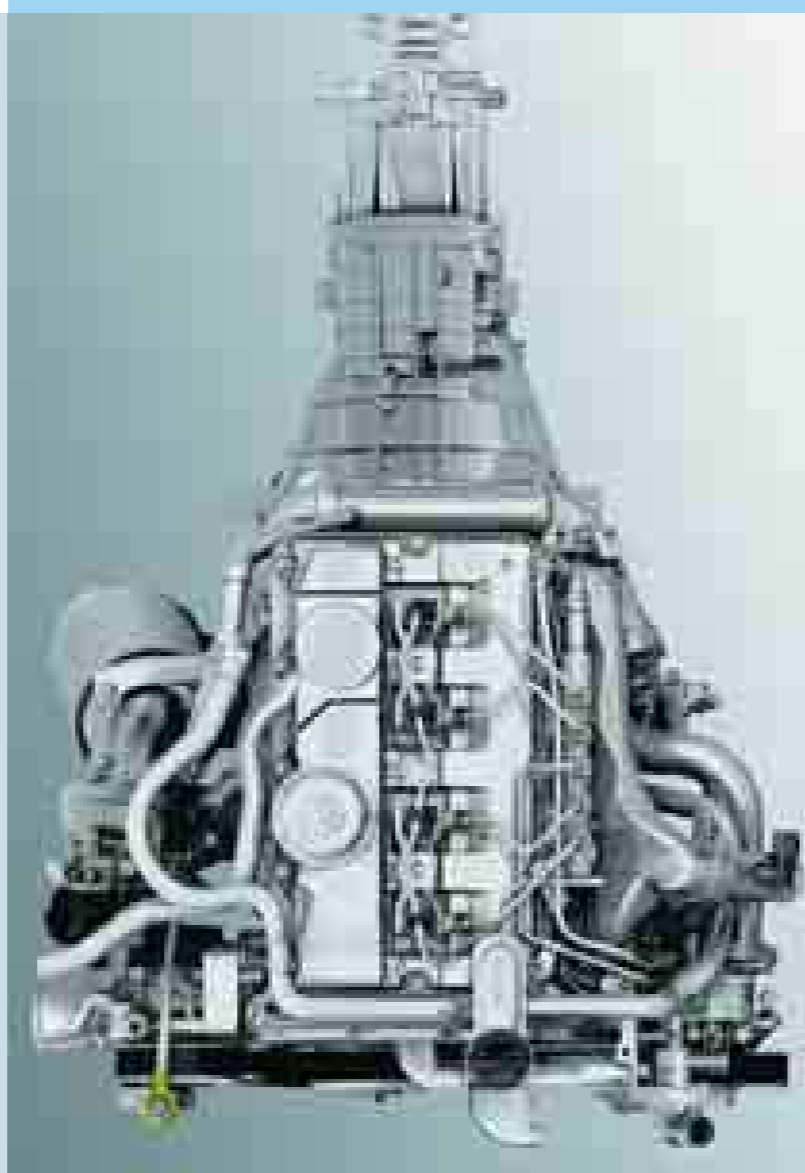
Rear-wheel drive Ford Transits are powered by a longitudinally-mounted 2.4 Duratorq TDCi diesel engine (above). Front-wheel drive models feature the new transversely-mounted 2.2 Duratorq TDCi diesel engine (left).
